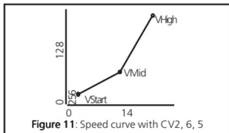
Figure 11: Speed curve with CV2, 6, 5
