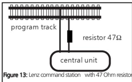
Figure 13: Lenz command station with 47 Ohm resistor
