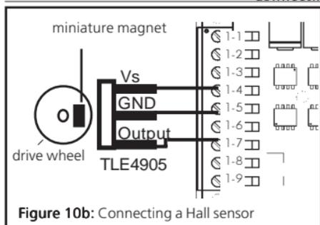
**Figure 10b:** Connecting a Hall sensor
