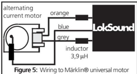
Figure 5: Wiring to Märklin® universal motor
