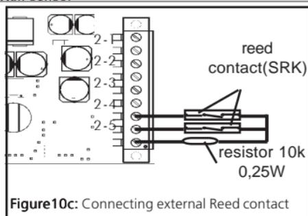
**Figure 10c:** Connecting external Reed contact
