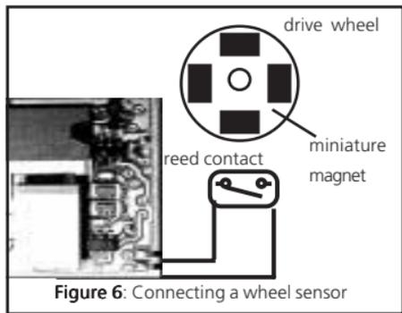
Figure 6: Connecting a wheel sensor
